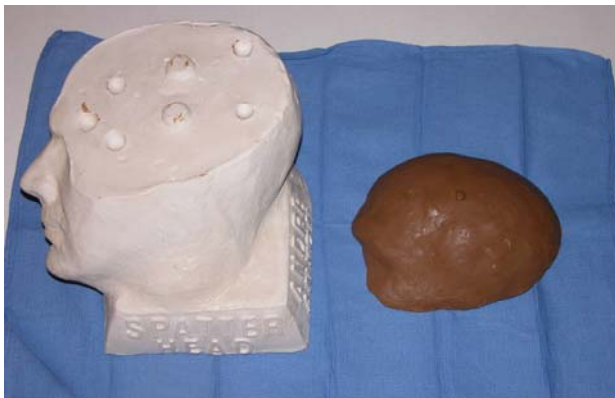
Figure 1. Spatter Head with blood-filled shell with pegs.
